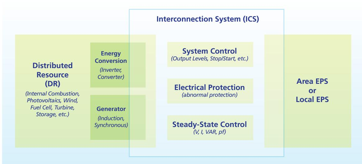
**Figure 2. The characteristics of an interconnection or point of common coupling for anti-islanding prevention as identified in IEEE 1547<sup>3</sup>.**
